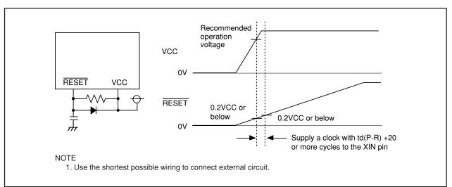
Figure 5.1 Example Reset Circuit
